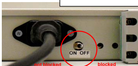
Figure 3 Blocking switch (device is in blocked condition)
