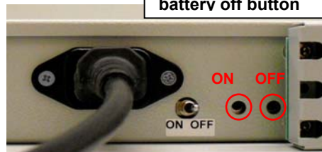
Figure 4 Battery on button and battery off button
