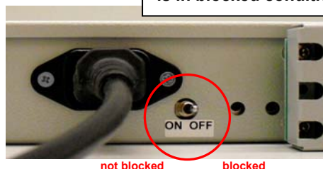
Figure 2 Blocking switch (device is in blocked condition)
