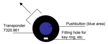
The 7320.962 transponder is equipped with two lines. These can be connected to a relay locking contact. Here, closing of the contact replaces the pressing of the blue pushbutton.
