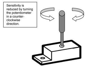
Sensitivity is increased by turning the potentiometer in a clockwise direction.
