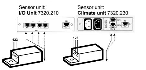
Pin assignment: Pin1: +48Volt Pin2: free Pin3: Ground
