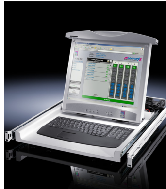
Monitor/keyboard unit, 17", native resolution 1280 x 1024
