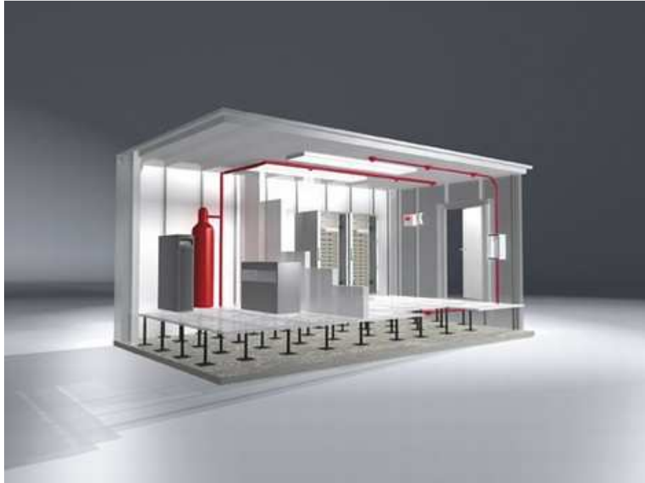
Illustration 9: IT safety space with extinguisher system
