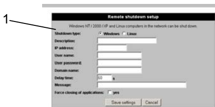
Fig. 23 Remote shutdown setup
